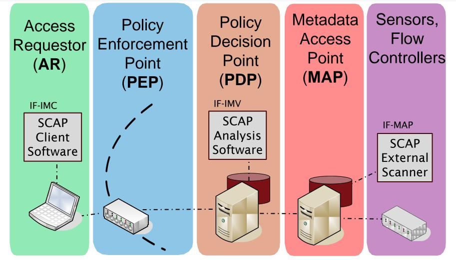
TNC handles the networking and network integration and SCAP handles compliance ---IF-IMC & IF-IMV designed for adding new device checks into TNC...
